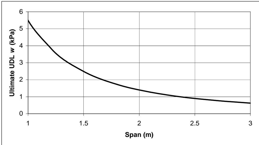
**Fig.9.2 Ultimate uniformly distributed load for simply supported Rapidwall® panels
