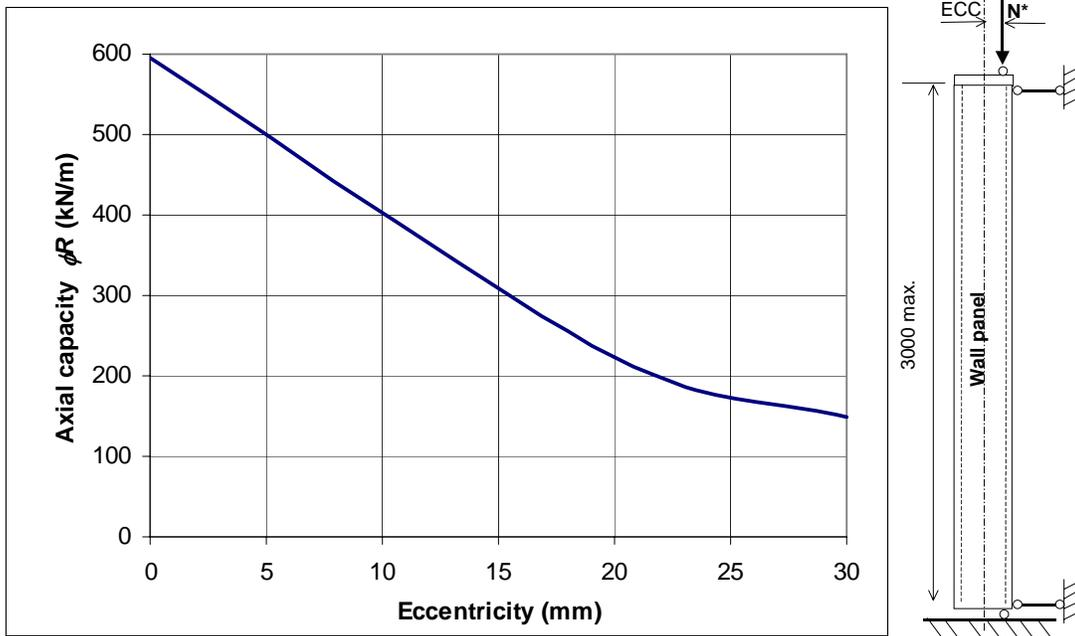
**Fig.11.2 Axial load capacity for concrete filled ( $\geq 25$ Mpa) Rapidwall<sup>®</sup> for all heights of walls  $\leq 3.0$ m – Both supports pinned**
