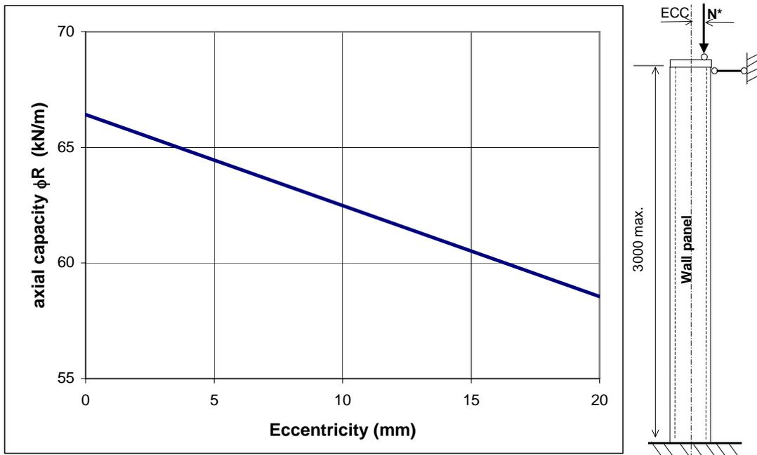
**Fig.11.1 Axial load capacity of unfilled Rapidwall<sup>®</sup> for all heights of walls  $\leq 3.0\text{m}$
