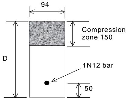
Fig. 10.4 Lintel cross-section for flexural strength calculation
