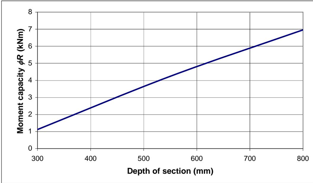
**Fig.10.2. Moment capacity of unfilled lintels**
