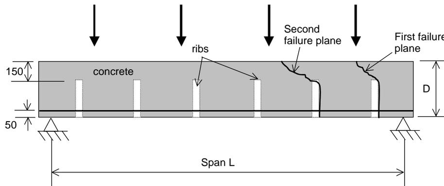
Fig.10.5 Typical shear failure mode
