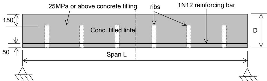
(b) Concrete Filled Lintel
