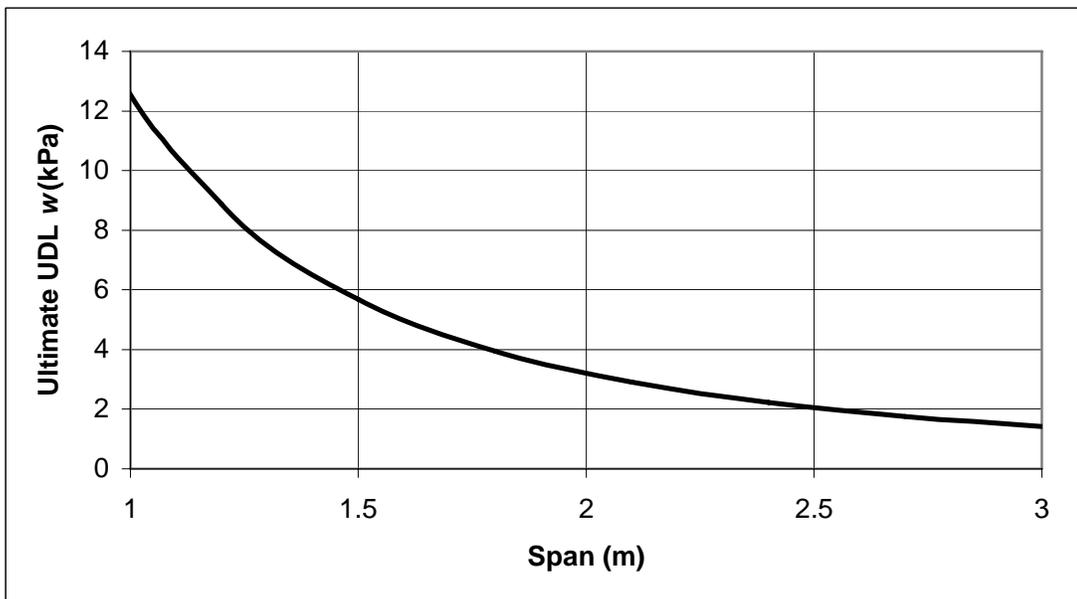
**Fig.9.1 Ultimate uniformly distributed load for simply supported Rapidwall® panels
