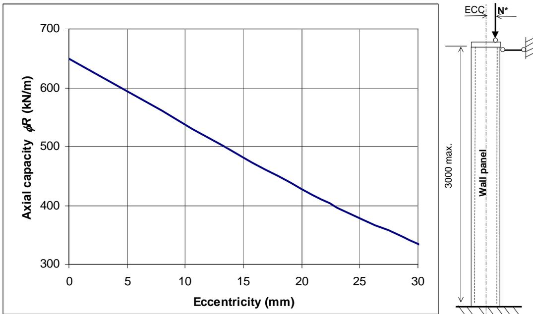
**Fig.11.3 Axial load capacity for concrete filled ( $\geq 25$ Mpa) Rapidwall<sup>®</sup> for all wall heights  $\leq 3.0$ m - one support pinned and one fixed**
