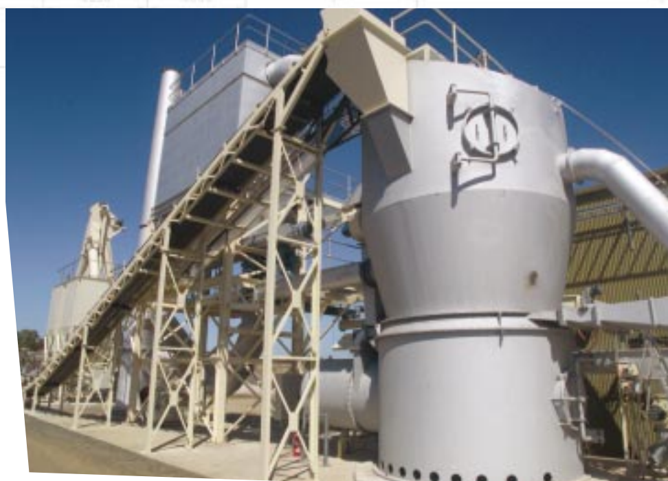
Ten tonne per hour Rapidflow Calciner Kilmore, Victoria, Australia
